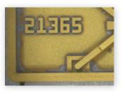
Silver may be visible in some areas on the interior of the package. This is acceptable as long as there remains complete gold coverage on the wire bond launch and the top surface of the exterior wall.
