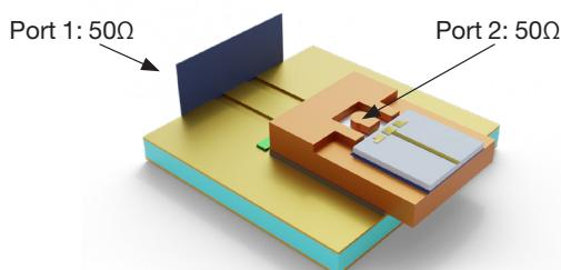
P1 is on the PCB with reference plane de-embedded to the edge of PolyStrata package. P2 is on the PolyStrata wire bonding pad. To approximate the wire bonds, an 80pH inductance is included in the plot for Return Loss and Insertion Loss (right figure).
