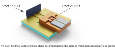
P1 is on the PCB with reference plane de-embedded to the edge of PolyStrata package. P2 is on the PolyStrata wire bonding pad. To approximate the wire bonds, an 80pH inductance is included in the plot for Return Loss and Insertion Loss (right figure).
