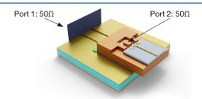
P1 is on the PCB with reference plane de-embedded to the edge of PolyStrata package. P2 is on the PolyStrata wire bonding pad. To approximate the wire bonds, an 80pH inductance is included in the plot for Return Loss and Insertion Loss (right figure).
