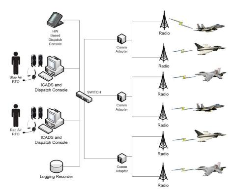
An Advanced Voice Communications System can be installed in each squadron and integrated with the ICADS to enhance pilot training. The radios are co-located with the live monitor equipment within the squadron and antennas are mounted alongside the RF data link antennas that communicate with the Airborne Subsystem (AS) pods. Analog audio from the radios is digitized and integrated into the ICADS network for monitoring and recording the live voice communications during live exercises.
