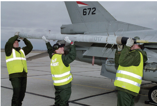
The mobile pods contain avionics that track and record aircraft events and position..
